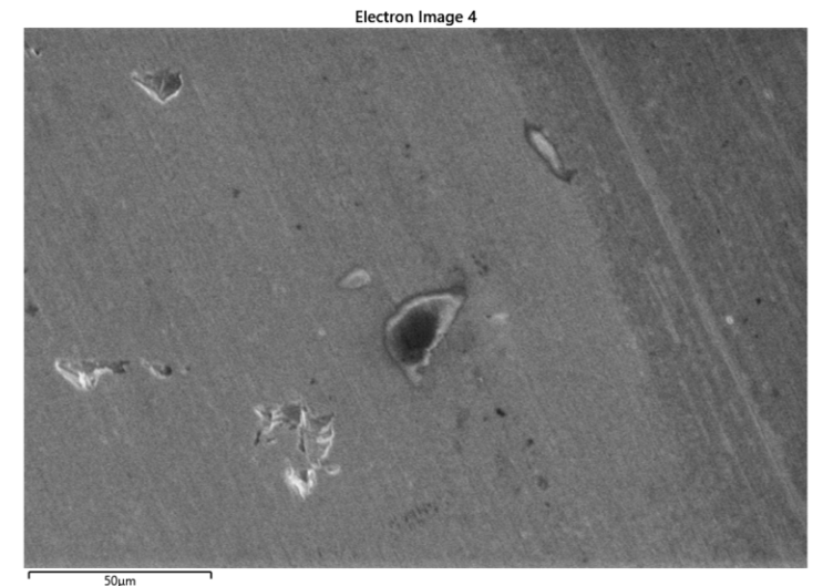
SEM-EDS map of YH1.9 specimen showing elemental map, showing small (~10 \mu\text{m} ) yttrium oxide particles in the YH matrix.
