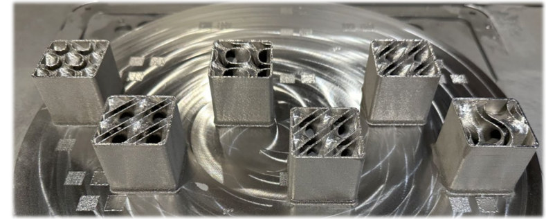
Sample 3-domain lattices produced specialized L-PBF process (INL with StarHagen LLC)
