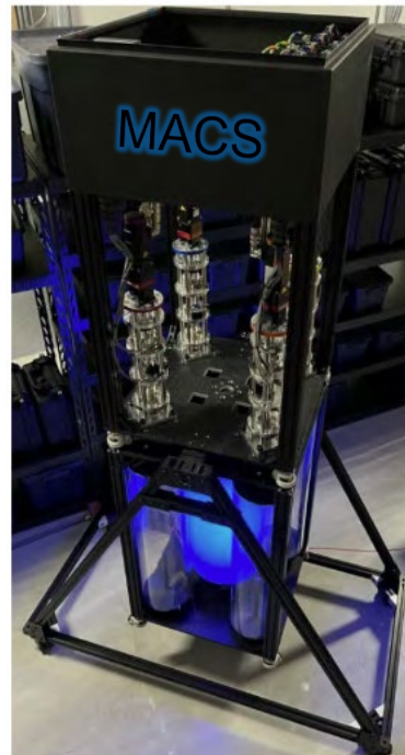
MACS Hardware (non-nuclear surrogate for MARVEL controls)
