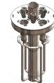
Primary Coolant Boundary Reactor Support Frame
