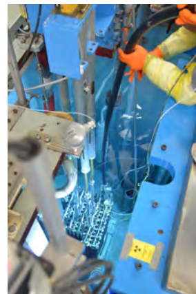
Fuel R & D - Irradiation of chloride-based HEU molten salt in NRAD
