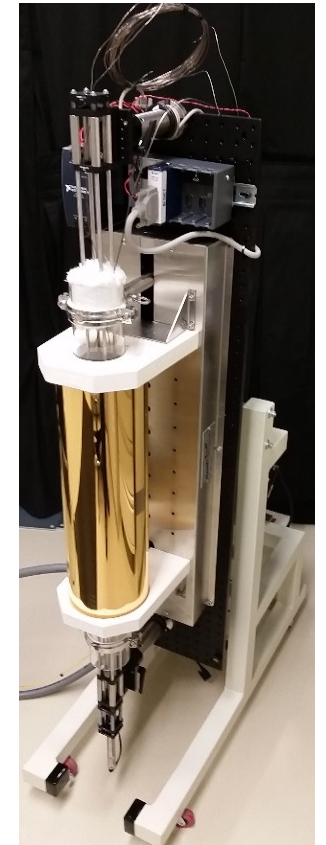
LVDT evaluations in horizontal and vertical tube furnace
