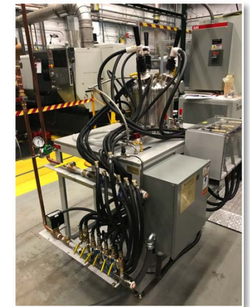
Arc-melter for alloy/compound preparation
