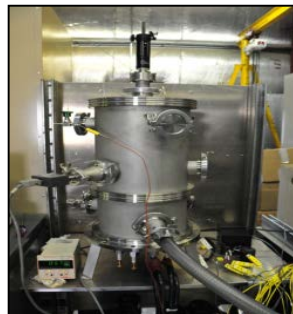
Fuel casting furnace in FASB (U capability in EFF)
