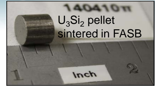
Fabrication development of accident tolerant fuel (U 3 Si 2 )
