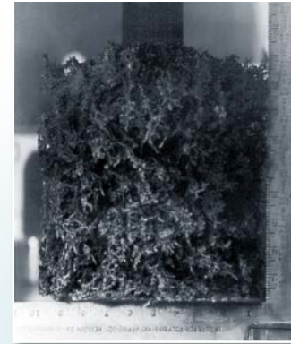
U metal recovered during fuel treatment
