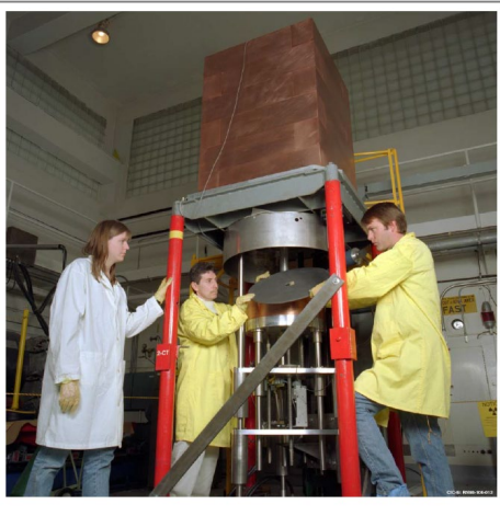
Comet: General purpose heavy duty vertical lift assembly
