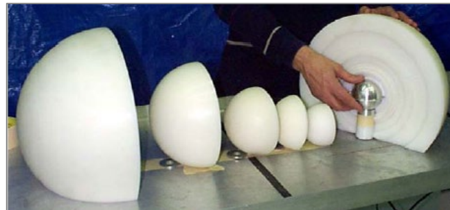
BERP Ball 4.5 kg alpha-phase Pu (94 wt% Pu-239)
