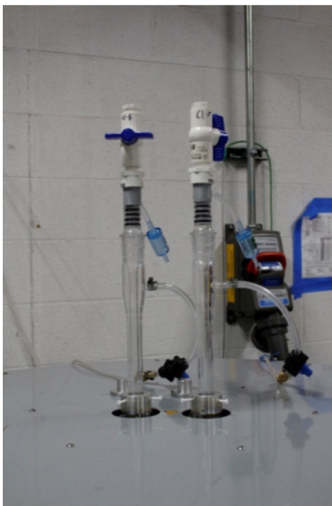
Figure 2-1. Two polyvinylchloride (PVC) ball valve droppers mounted onto the glassware of the Setaram AlexSYS-800 drop calorimeter.
