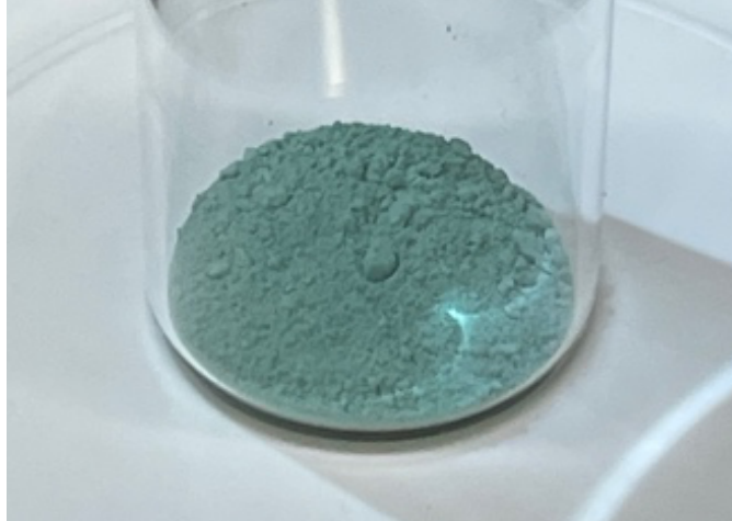
Figure 2-1. \text{UF}_4 synthesized using non-hydrofluorination processes.
