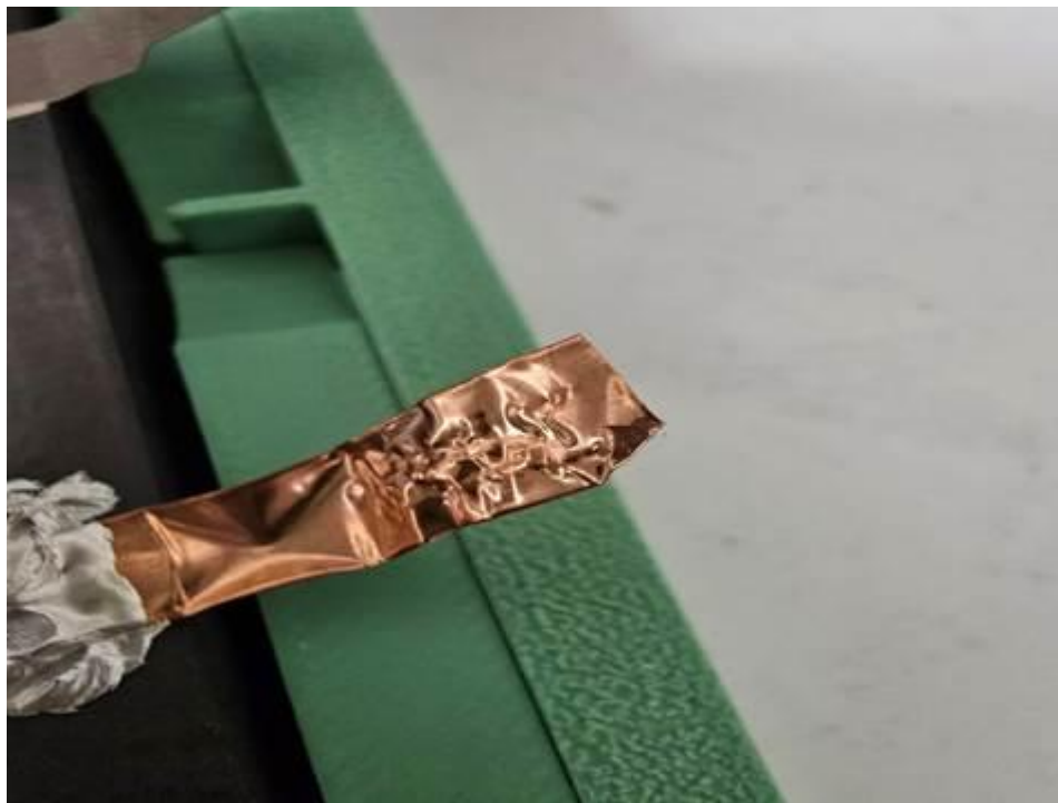
Figure 9. Physical deformation of a copper tape electrode.
