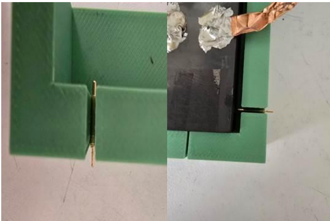
Figure 3. (a) Single spring-loaded pin located in fixture shell and (b) single spring-loaded pin location on graphite sample surface (with retaining ring removed).
