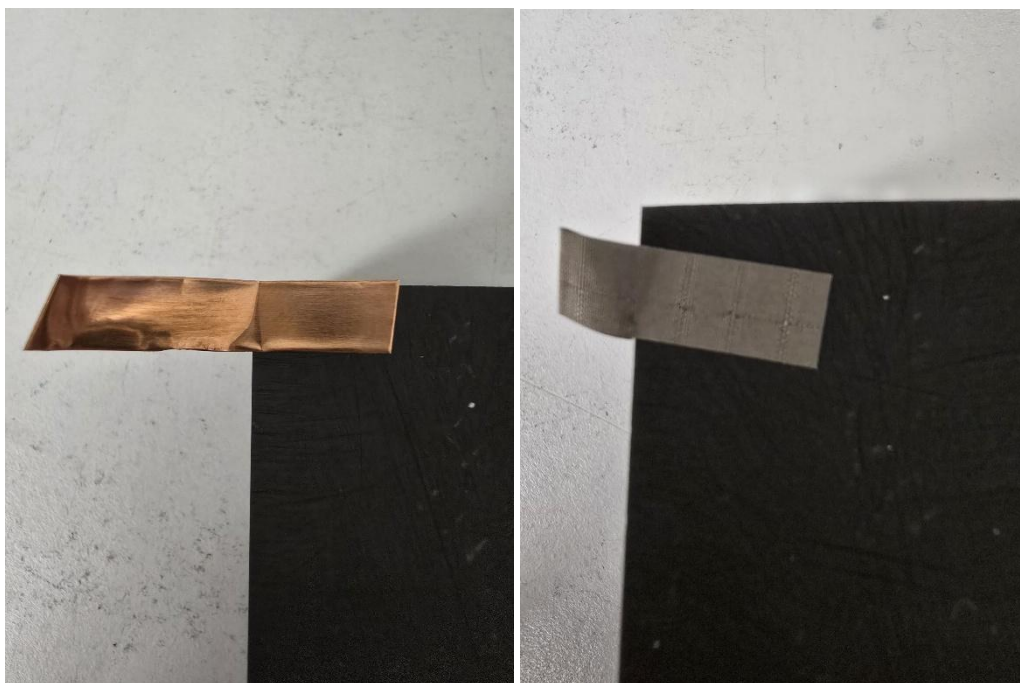
Figure 6. (left) Copper tape and (right) conductive fabric tape adhered to the surface of the graphite sample.
