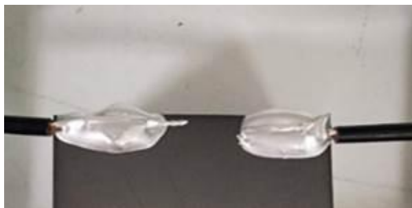
Figure 5. Copper wire adhered to graphite surface with silver epoxy.
