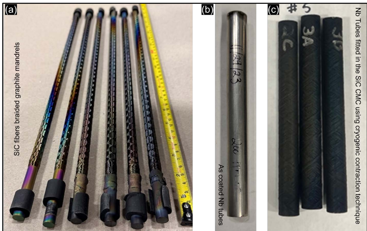
Figure 4: (a) SiC fibers braided graphite mandrels (~50 cm long) after going through the process pyrolytic carbon coating to generate a layer of carbon over the fibers for better bonding with PIP SiC matrix. Picture credit CTP LLC. (b) 10 cm long, as coated Nb tube sections shipped to CTP & (c) 10 cm long coated Nb tubes shrink fitted within SiC CMC shells.
