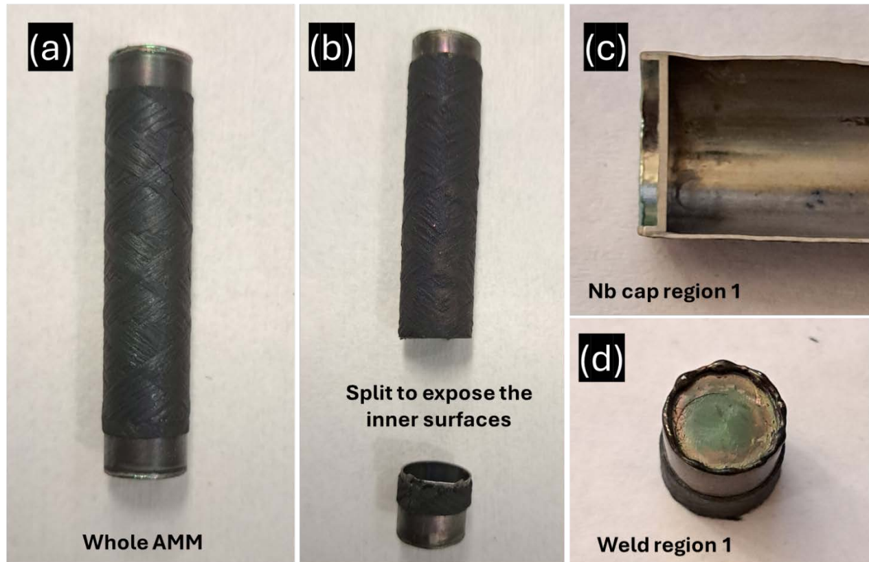
Figure 22. Optical images of the AMM module with multilayer-coated Nb cap region ( 2 \times 300 nm Al 2 O 3 + 2 \times 300 nm Cr). (a) Whole AMM module following thermal testing, (b) split AMM exposing intact inner surfaces, (c) Nb cap region showing slight discoloration, and (d) weld region highlighting surface features following exposure.
