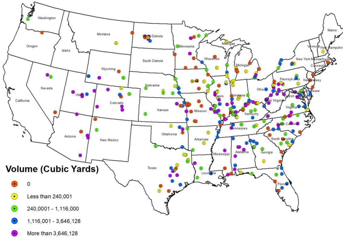
Figure 3-3. Quantity of CCR and, if applicable, water held in the unit as of 2020/2021. The data was accessed at EarthJustice (2022b).
