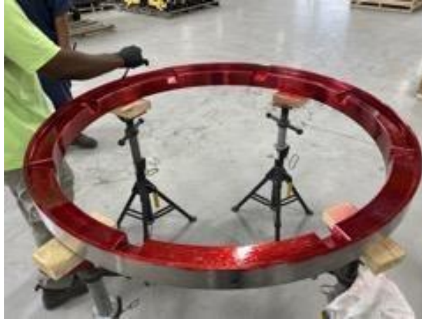
Figure 12. The plenum support ring was machined from billet 316H forging material (ASME SA182), requiring 100% liquid penetrant examination per Section III.
