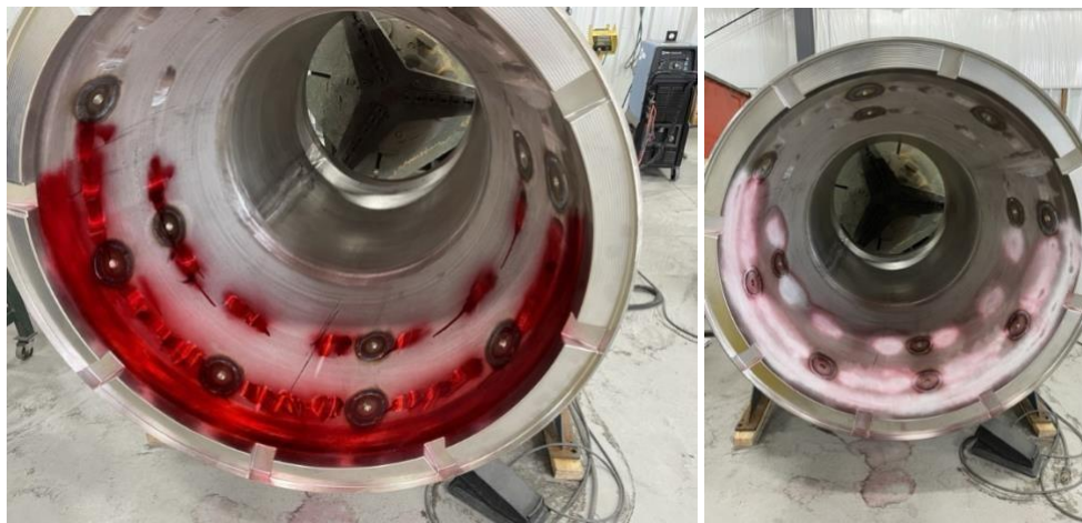
Figure 13. Dye penetrant inspection following the removal of temporary attachments.
