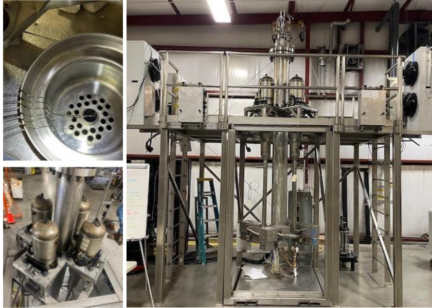
Figure 19. MARVEL assembly and setup at Creative Engineers Incorporated (CEI), including (top left) TC wires inside heat exchanger, (bottom left) Stirling engines installed, and (right) PCAT assembled and setup at CEI (without insulation).
