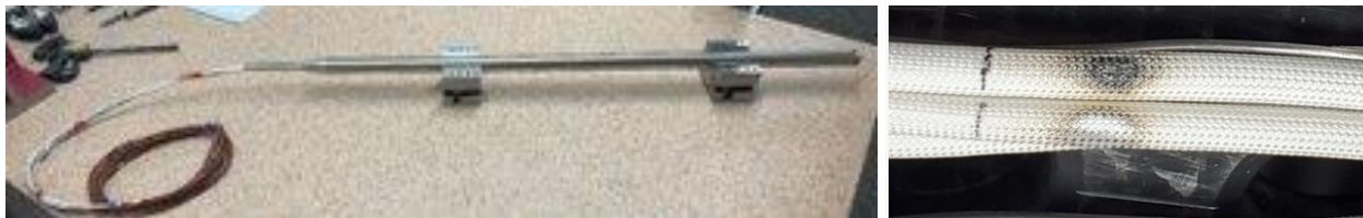
Figure 16. (Left) PCAT heater tube and cartridge heater pigtail and (right) heater insulation damage due to end cap welding.
