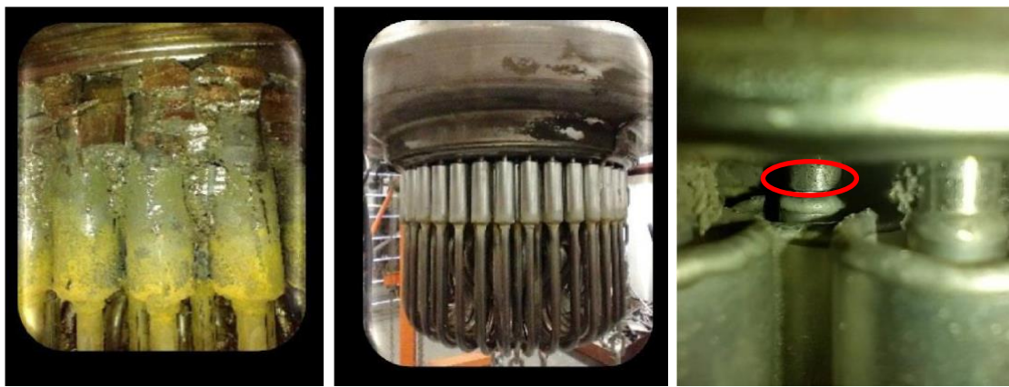
Figure 21. Images showing (left) oxide build-up on Stirling engine HX tubes, (center) Stirling engine HX tubes after cleaning, and (right) Stirling engine HX tube failure.
