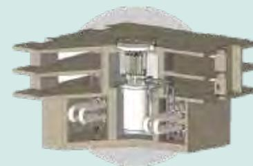
The eVinci™ Micro Reactor uses TRISO fuel and is designed for transportability to reduce construction costs and eliminate the need for waste and spent fuel storage on site. The DOE will pay \$7.4 million towards the \$9.3 million cost.
