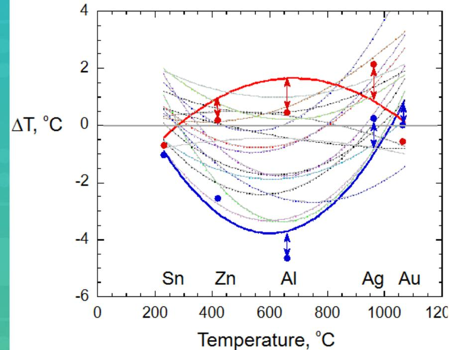
Residuals for known and fit temperatures for each reference material in calibrations spanning six years
