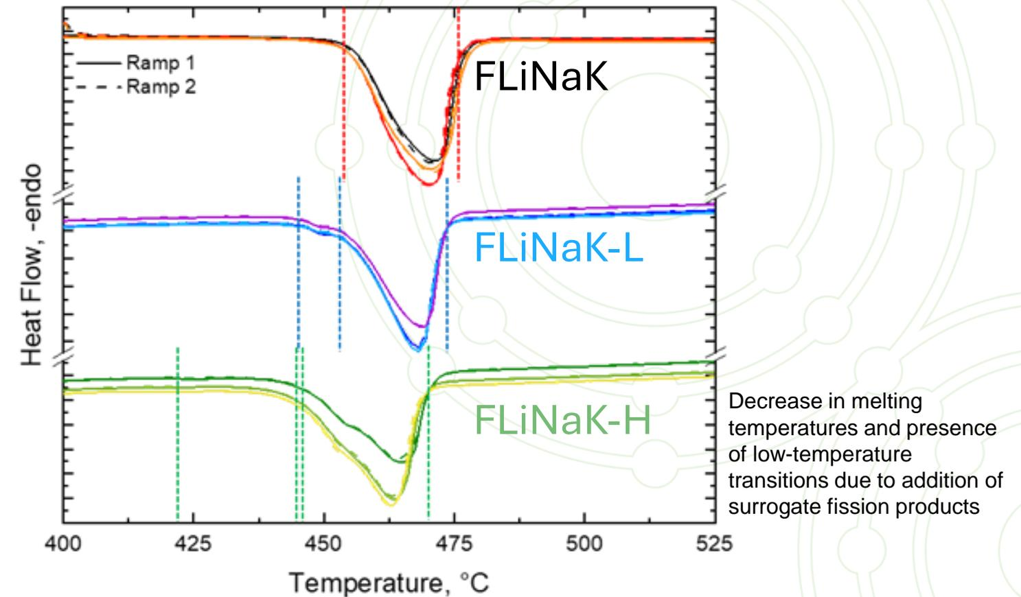
**Lower onset of melting and liquidus point temperatures were measured for both low-burnup FLiNaK and high-burnup FLiNaK compared to those of pure FLiNaK, for which the onset of melting and liquidus point temperatures were 455 °C and 476 °C, respectively**
