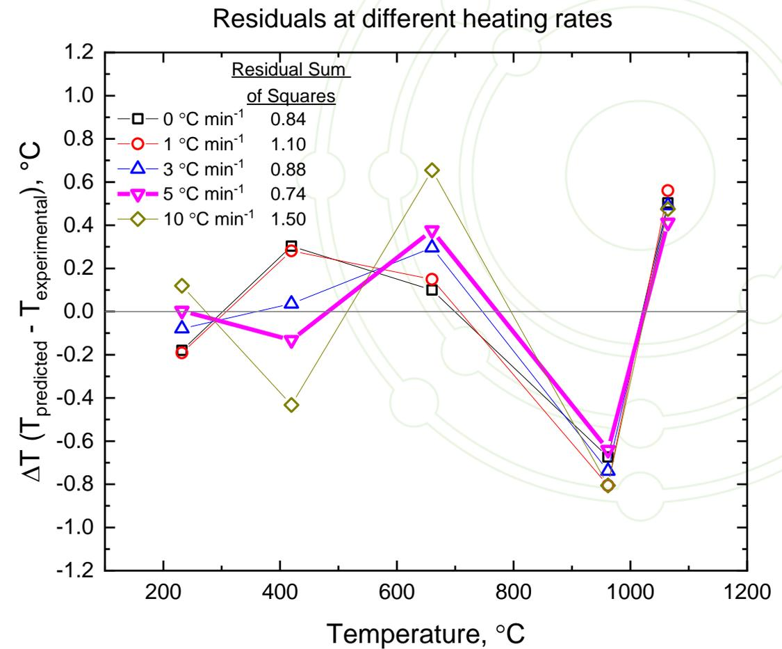
**Effect of heating rate was investigated by recording DSC responses of five reference metals at heating rates of 1, 3, 5, and  $10\text{ }^{\circ}\text{C min}^{-1}$  and extrapolating to  $0\text{ }^{\circ}\text{C min}^{-1}$ .**
