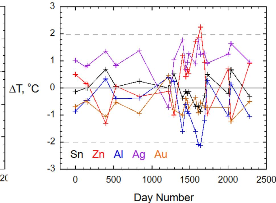
**Both the precision and accuracy of calibration curves are within 2 °C over this time span and temperature range**
