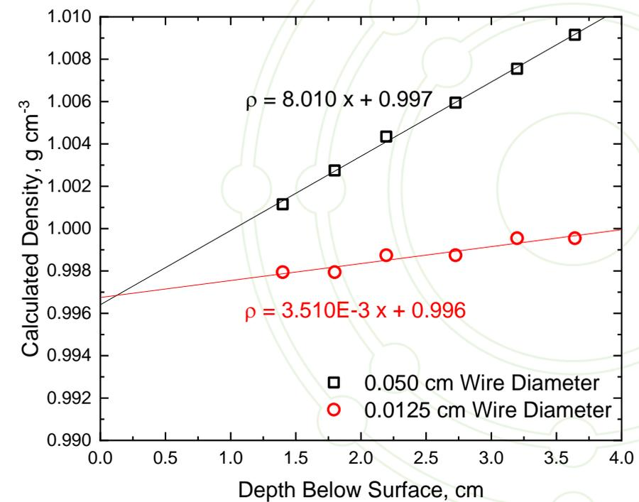
Density of water measured with two different wires and the same bob at different immersion depths
