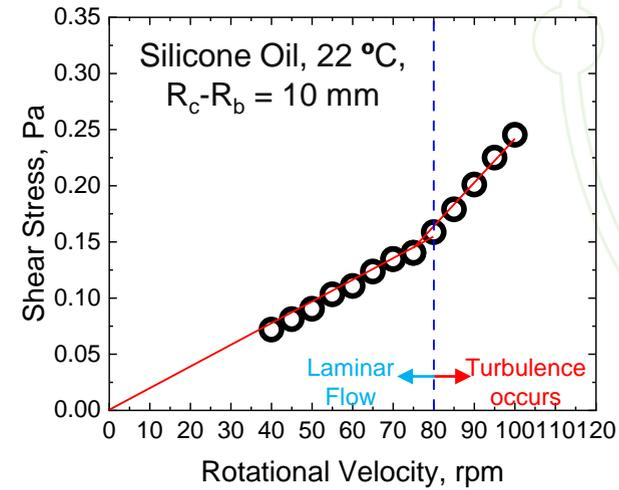
Laminar flow is maintained by using a cell having a narrow gap between spindle and crucible walls.
