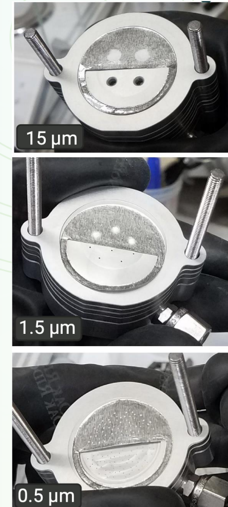
Cascade Impactor - Measuring aerosol sizes over halide salts
