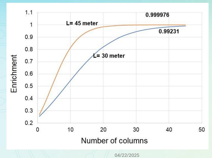
Enrichment in <sup>37</sup>Cl for 30-m and 45-m columns using  $\alpha$ and L (the column length) as chosen and transport calculated from data described above
