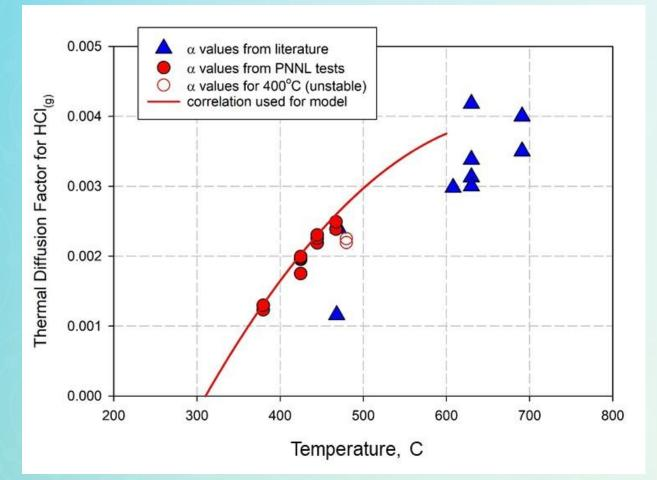
Comparison of PNNL and literature value measurements of the thermal diffusion constant,  $\alpha$ , for HCI<sub>( $\alpha$ )</sub>. The temperature plotted is the T<sub>avg</sub> of the column.
