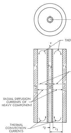
The separation column for TDIS is a tube inside of a tube, where thermal convection currents and radial diffusion work to provide the isotope separation.
