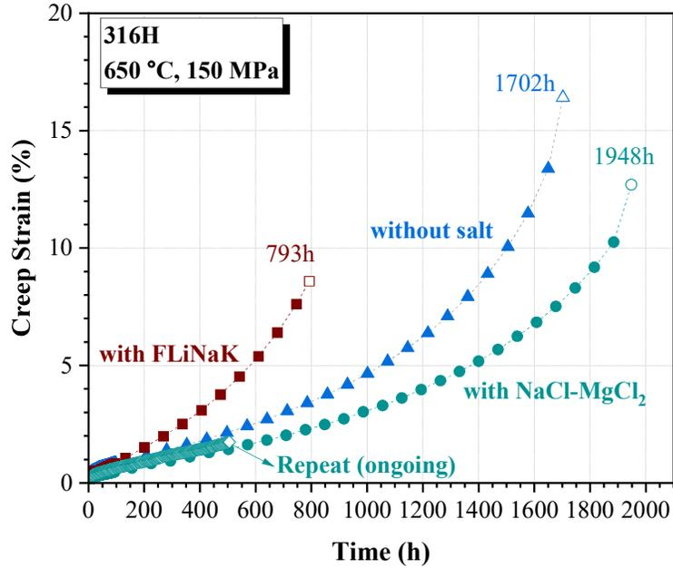
Figure 1: Measured creep strains of 316H in air, FLiNaK, NaCl-MgCl<sub>2</sub> at 650°C/150 MPa. Open symbols indicate failure time.
