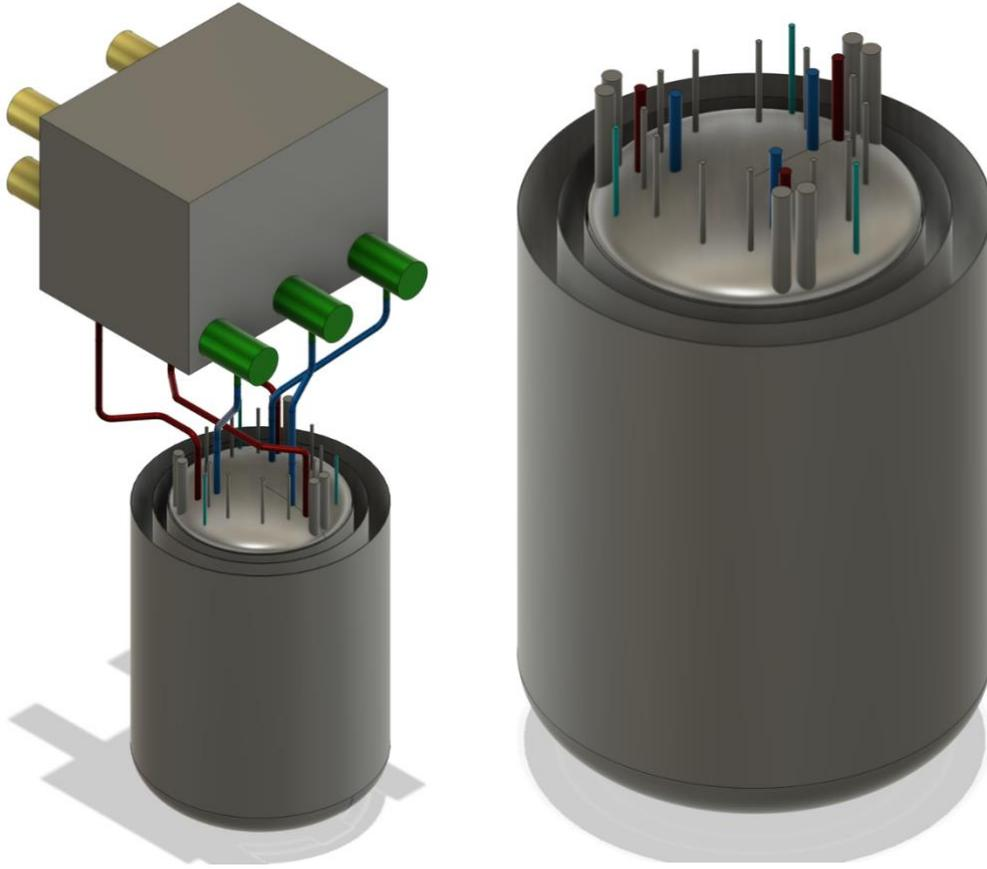
Figure 15. *Left:* zoomed-in view of the reactor and IHX, with pumps in green and pipes into the balance of plant container in yellow. *Right:* Zoomed-in view into the reactor, showing the multiple vessels responsible for the RVACS, sodium guard vessel, and main vessel, with pipe and pump shaft penetration. Red pipes are the hot side, blue pipes the cold side.
