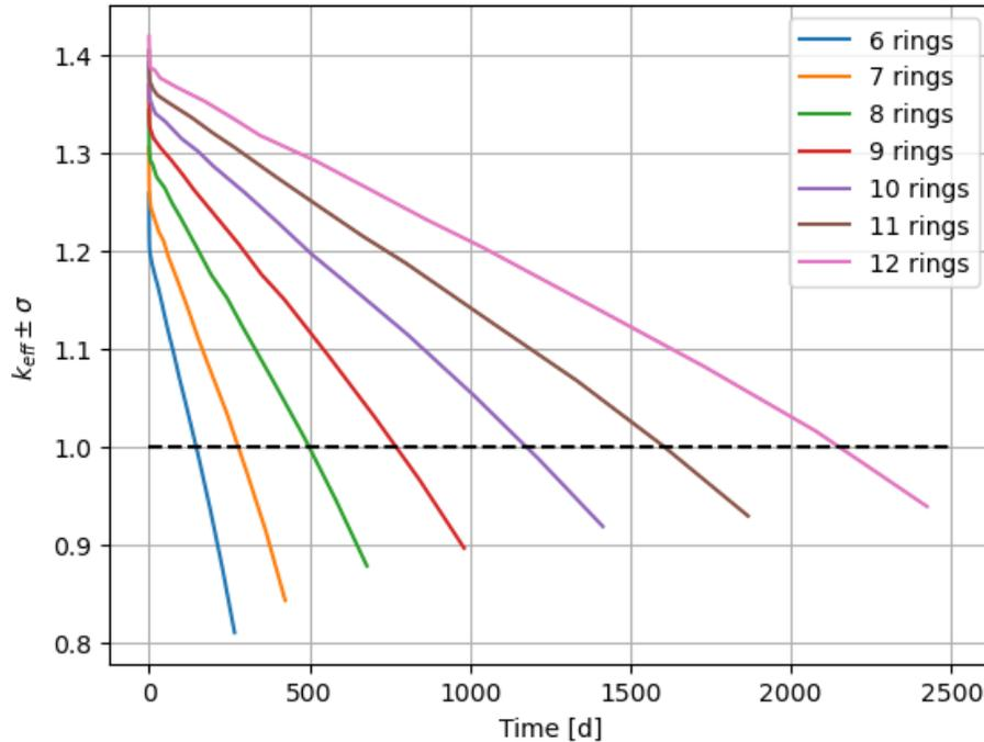
Figure 4. Parametric study of operational time by varying the number of rings in the core.
