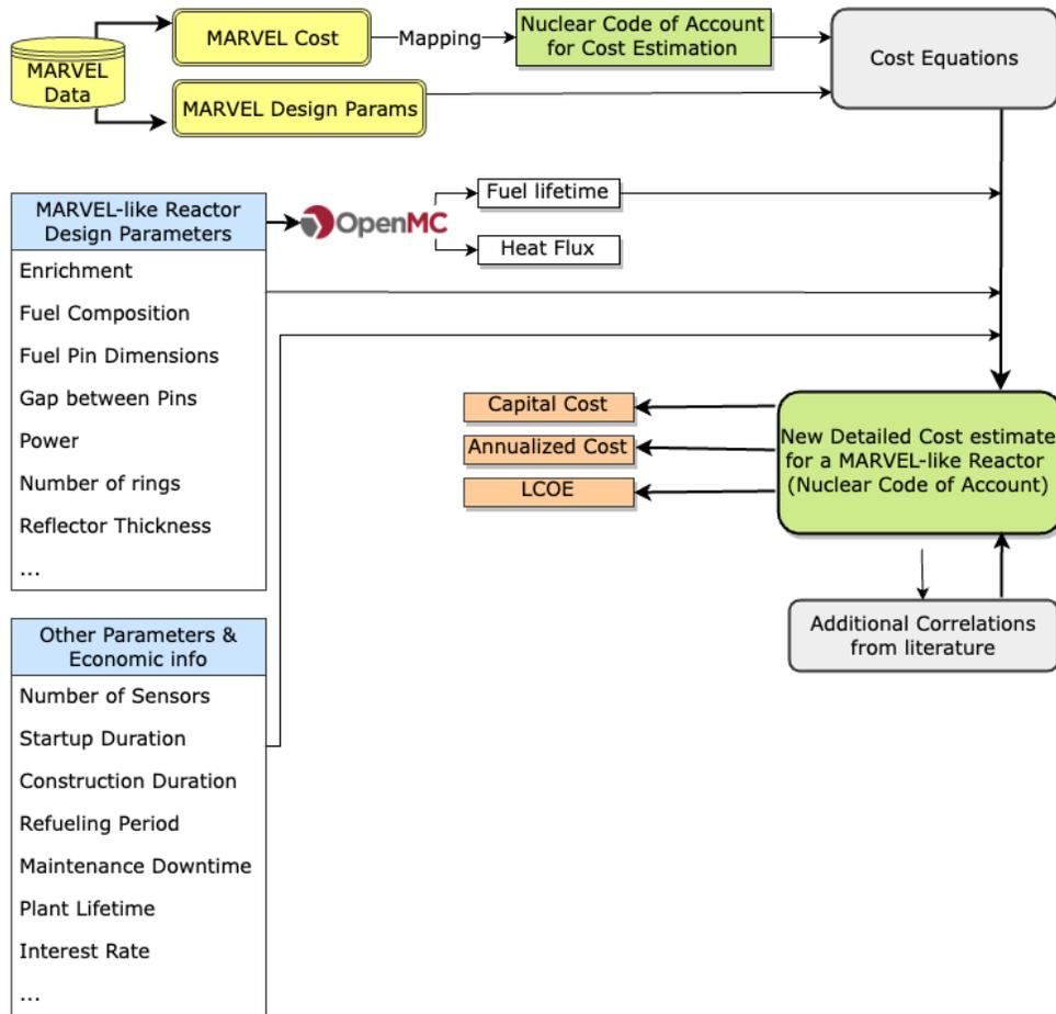
Figure 23. Neutronics-Economics Framework: Leveraging the MARVEL microreactor project data and coupling OpenMC (neutronics) with cost equations (economics) to estimate the capital cost, annualized cost, and LCOE of an LMTR reactor.
