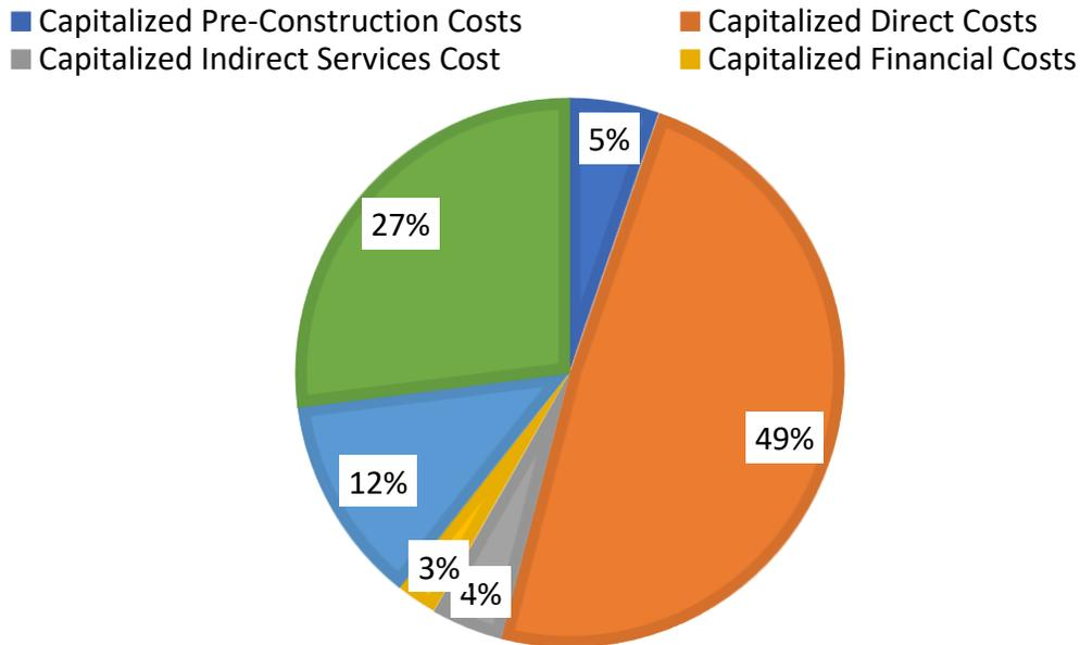
Figure 28 LMTR-20 NOAK levelized Cost (\$/MWh) Breakdown. The contribution of each cost to the LCOE is presented as a percentage.
