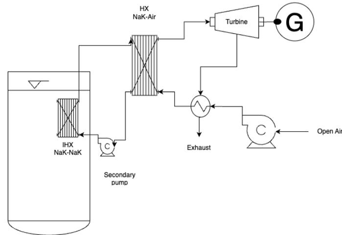
Figure 13. Sketch of the heat transfer loops and power block.
