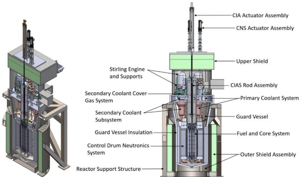
Figure 2. MARVEL microreactor cutaway view. Taken from (Gerstner and Arafat 2023). CIA stands for the central insurance absorber
