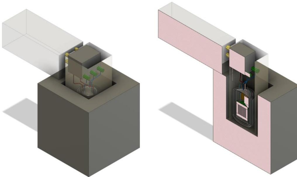
Figure 14. System overview with concrete base and separate containers (*left*) and cross section (*right*) of the system showing the reactor below grade inside the concrete pit. Not all dimensions are final or to scale.
