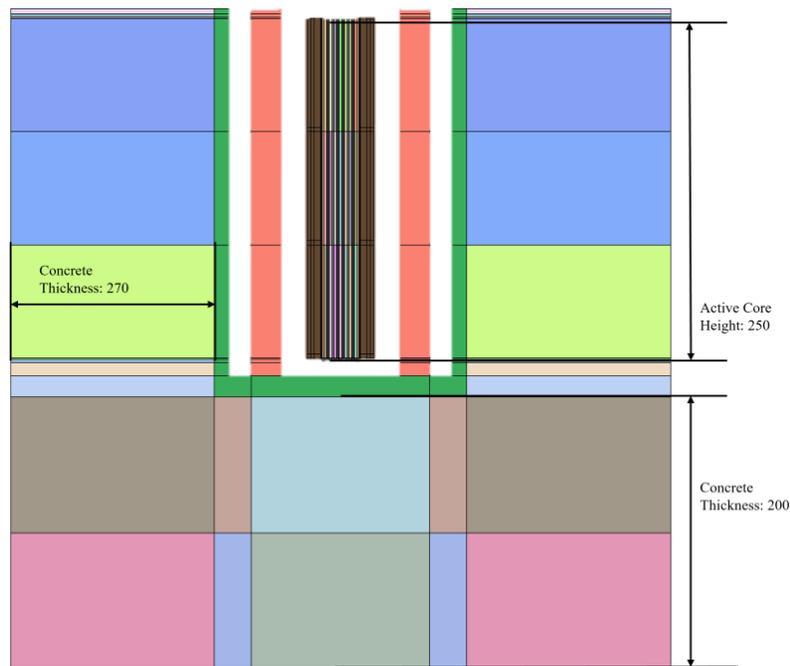
Figure 6. Dimensioned axial cross-section of the LMTR core in cm.
