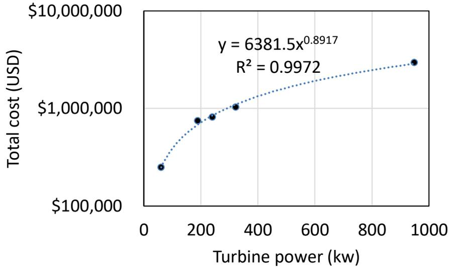
Figure 19. Microreactor turbine cost vs. turbine power.
