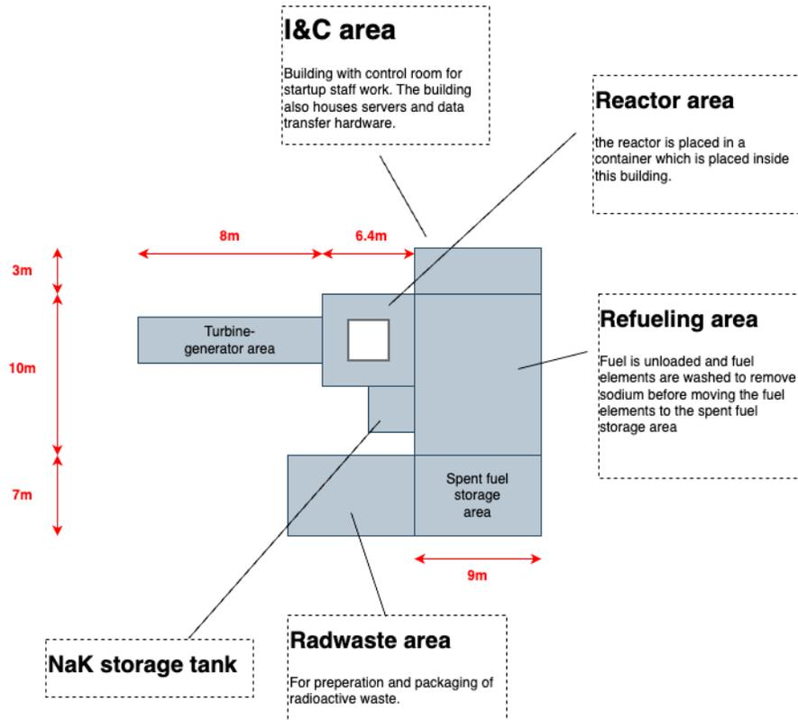
Figure 18. Suggested plan layout and area dimensions.
