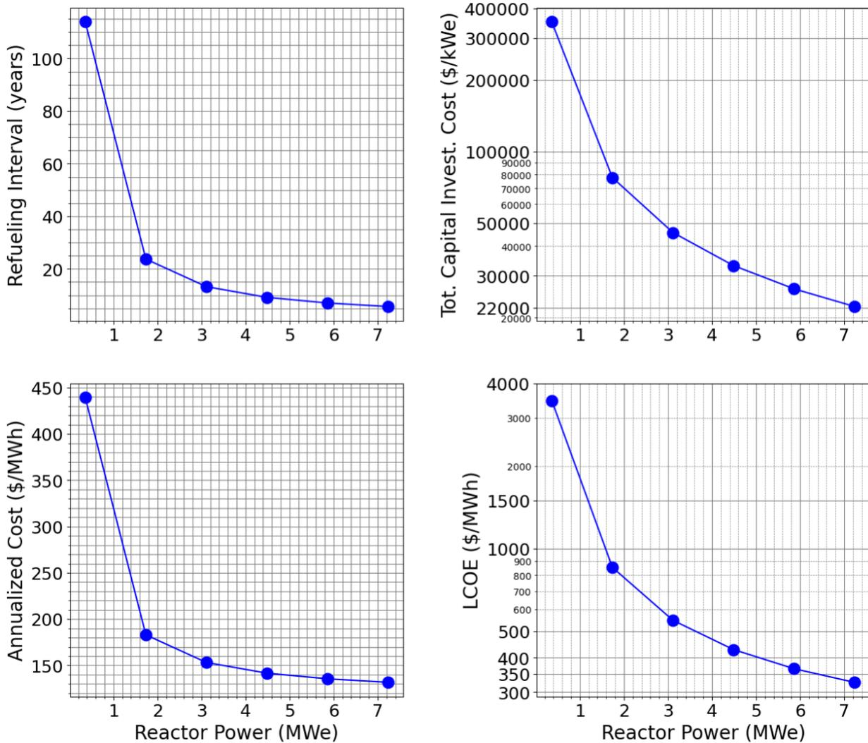
Figure 24. Economic figures of merit dependence on the reactor power.
