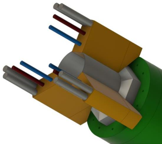
Figure 17. Zoomed-in view of the core heat exchangers and the baffles that separate the hot and cold side of the fluid domain.
