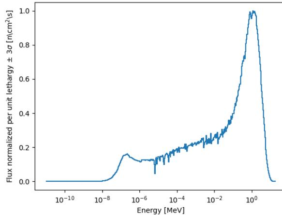
Figure 7. Hardened thermal spectra of an LMTR core.
