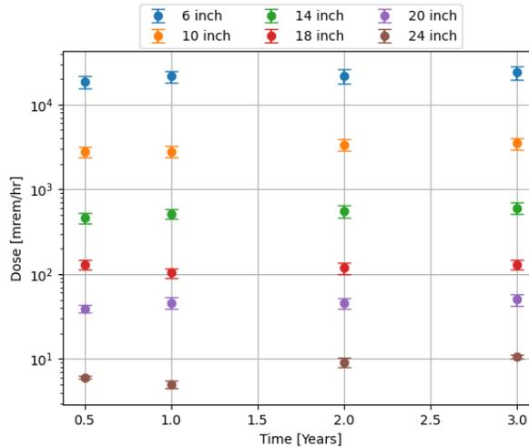
Figure 9. Dose 30 cm above pit for several thicknesses  $\pm 3\sigma$ .
