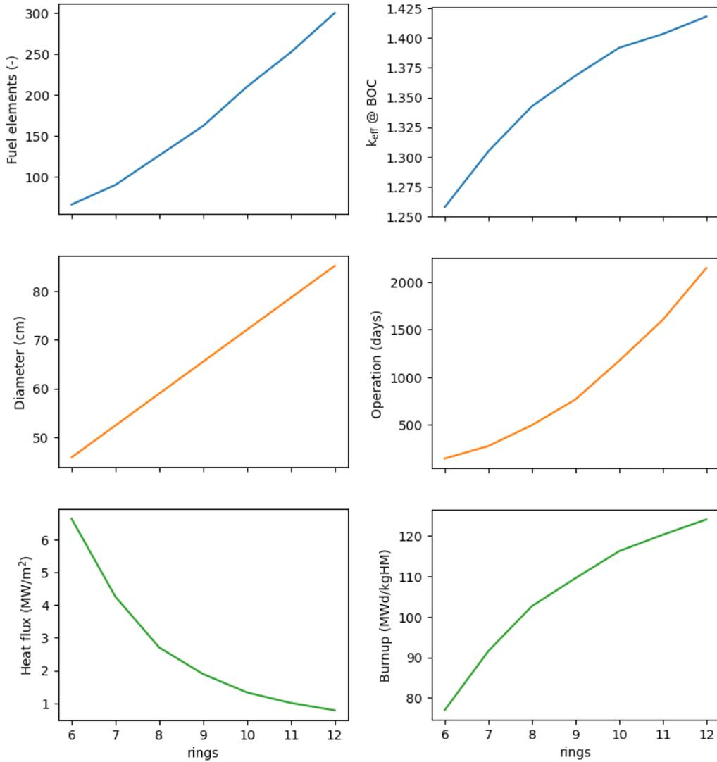
Figure 5. Parametric study of various quantities by varying the number of rings in the core. BOC stands for Beginning of the fuel cycle.
