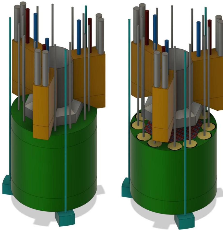
Figure 16. Reactor core with and without top reflector for exposition.
