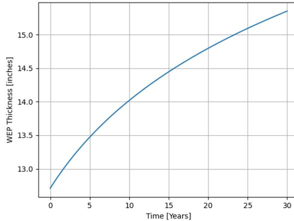
Figure 12. Required WEP thickness as a function of core lifetime.
