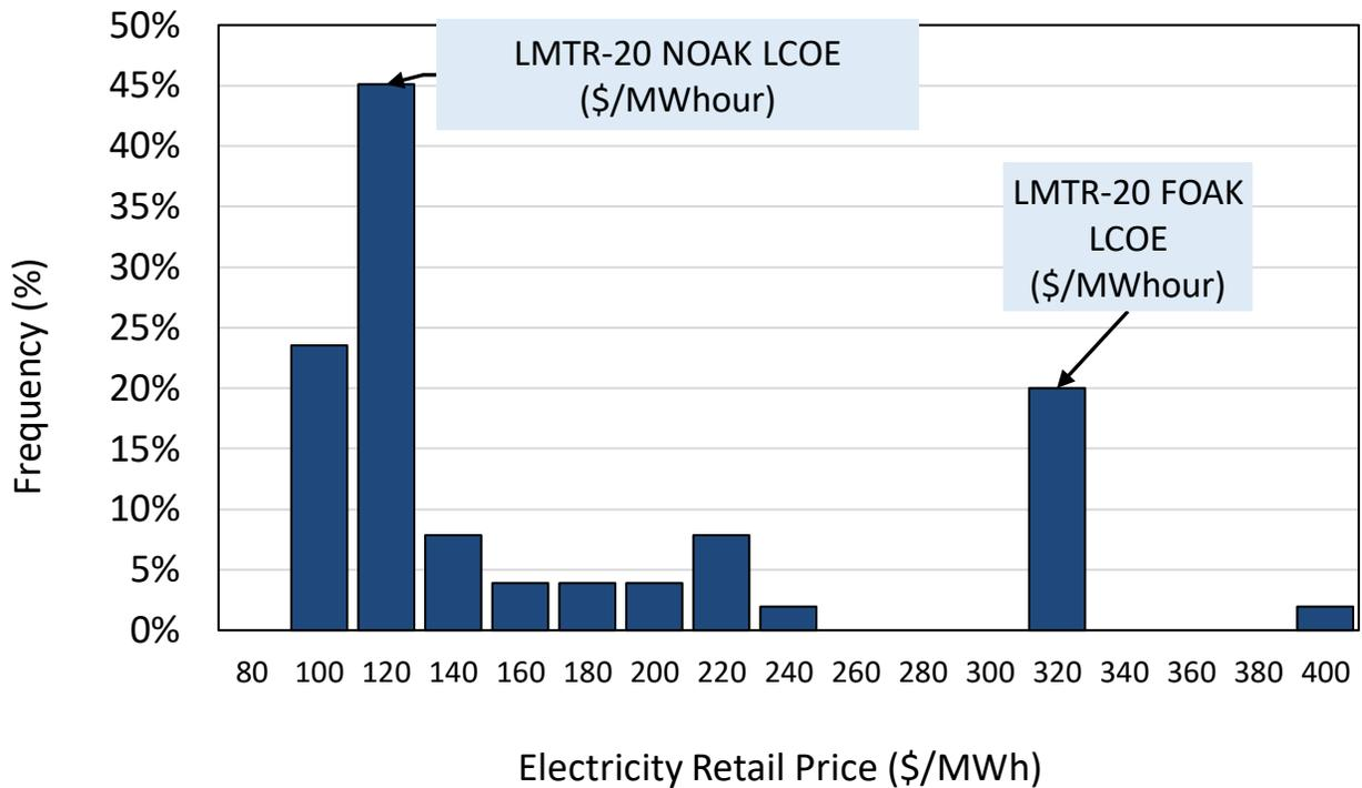
Figure 27. The LCOE of the LMTR-20 FOAK and NOAK reactor compared to the retail electricity price distribution.
