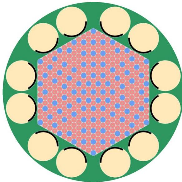
Figure 3. 2D view of the core lattice arrangement. The red circles are the TRIGA fuel pins. The blue circles are the moderator pins (zirconium hydride). The outer 12 circles are the CDs (beryllium in yellow and boron carbide in black). The outer green area is the BeO reflector.
