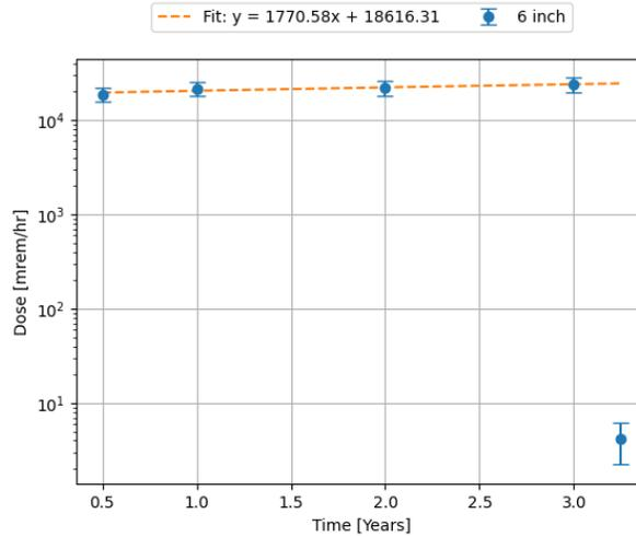
Figure 10. Dose 30 cm above the pit for 6-inch-thick WEP with decay dose rate,  $\pm 3\sigma$  plotted.
