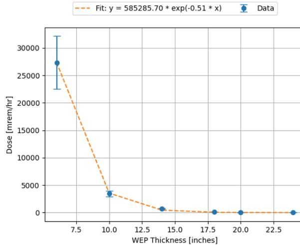
Figure 11. Dose rate immediately after shutdown as a function of WEP thickness,  $\pm 3\sigma$  plotted.
