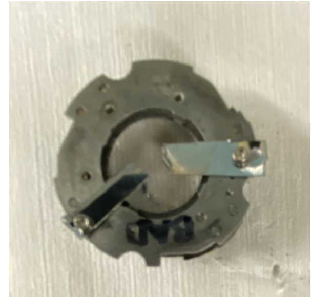
Ytria powder cathode and new high temperature stage commissioned at UTK
