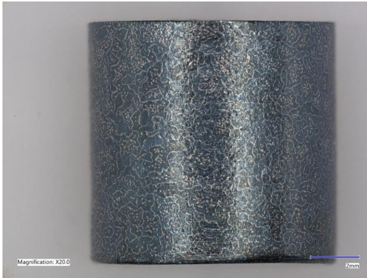
YH1.5 sample: spinel-type structure
