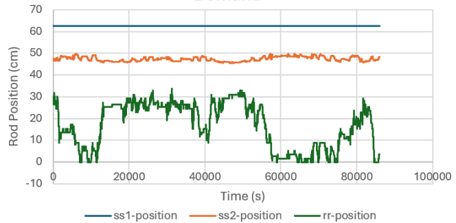
Load Following Control Rod Movements - Cos Demand
