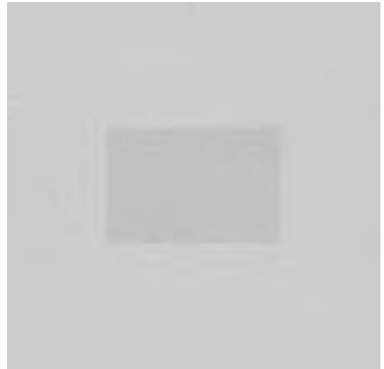
Figure 8. Grayscale representation of the number of neutron captures in a scintillator behind the object in Figure 7.
