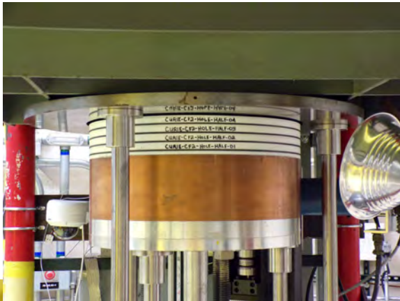
CURIE: Uranium and Teflon to test unresolved resonance region.
