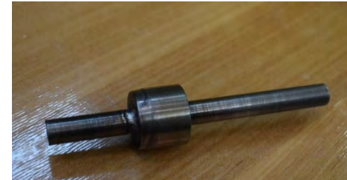
Heat Pipe Condenser Plug with Fill Stem Before Cleaning
