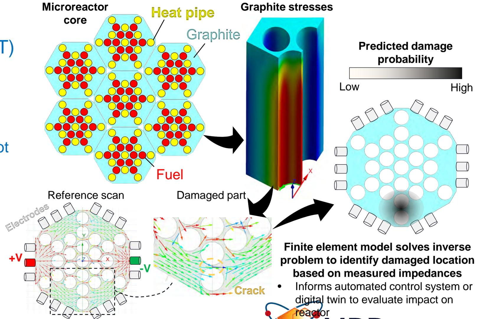
**Current paths during measurements of impedances between electrode pairs**
