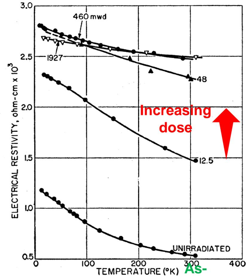
**Evolution in electrical resistivity under neutron irradiation**
