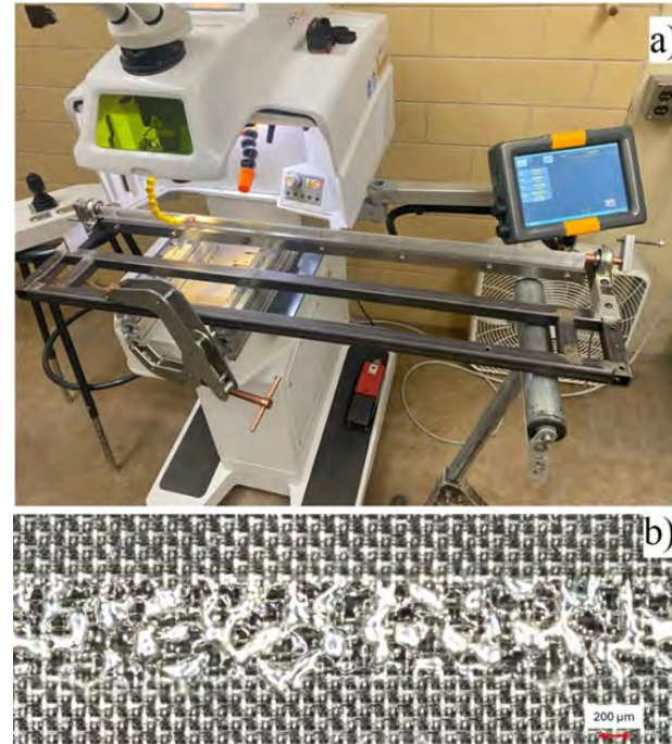
Figure 3. a.)Laser weld station, b.)Microscope image of laser weld .
