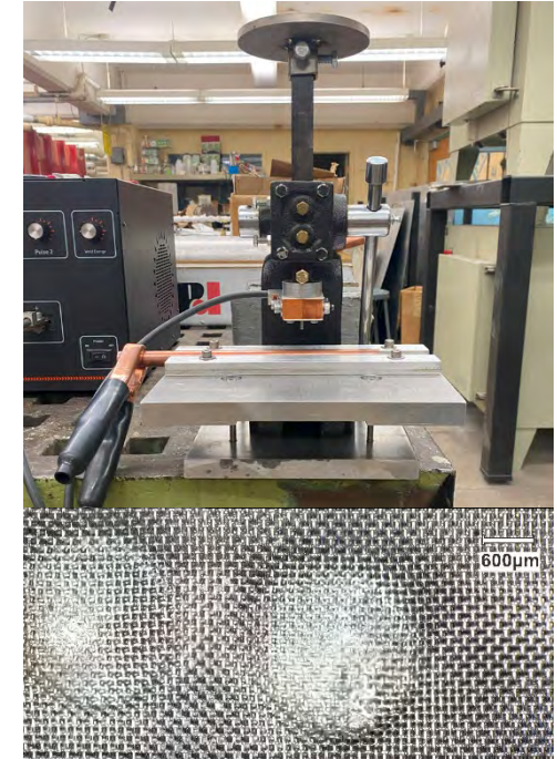
Figure 4. a.)Diffusion bond station, b.)Microscope image of bond.
