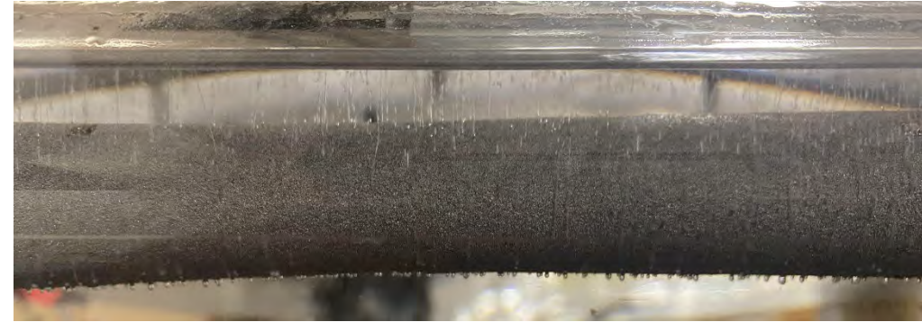
Figure 6. Porous sintered tube wick bubble test.
