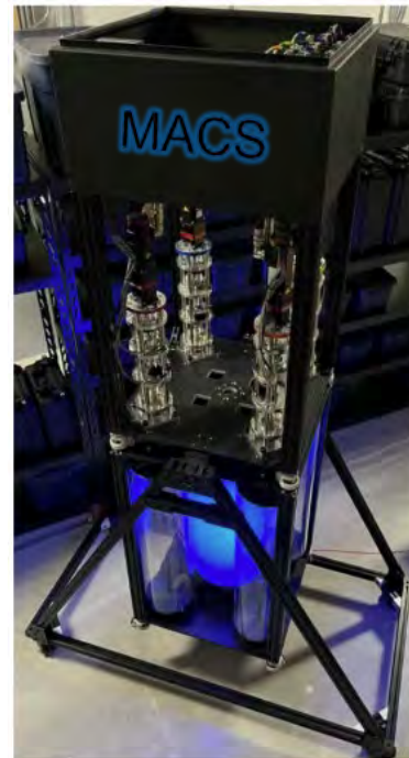
MACS Hardware (non-nuclear surrogate for MARVEL controls)
