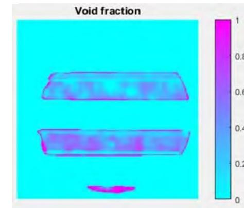
X-ray images showing higher Void in the wake zone below the Heater tubes
