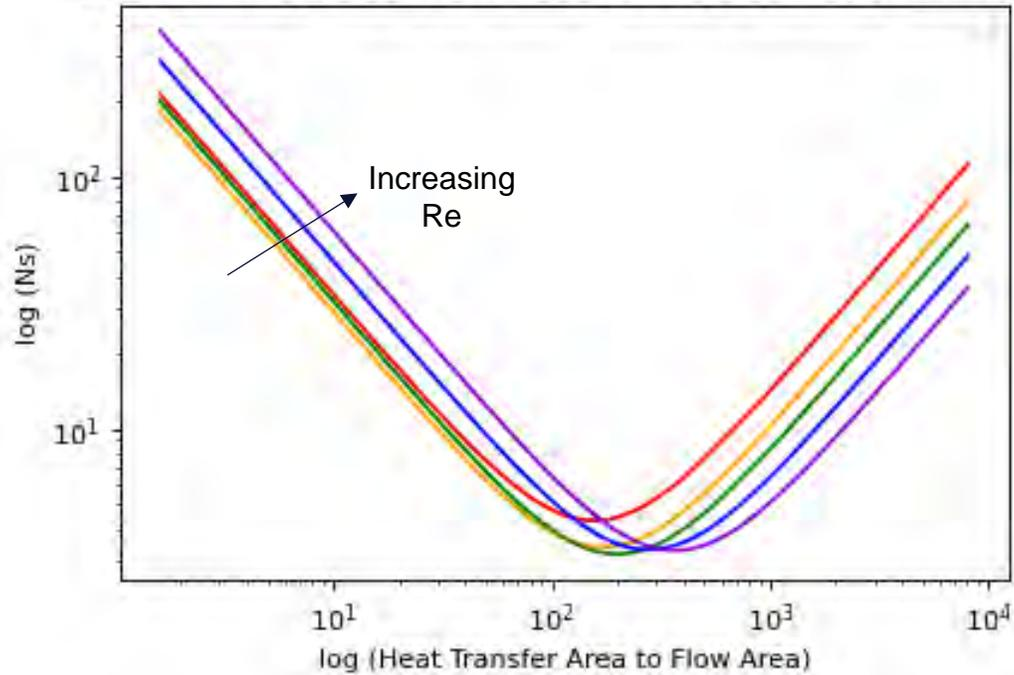
Entropy Generation Rate of Cross-flow HX at with Primary side (Na-K Heat pipe) & Secondary fluid (Particles)
