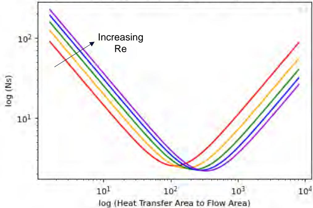
Entropy Generation Rate of Counter-current HX at with Primary side (Helium) & Secondary fluid (Molten Salt)
