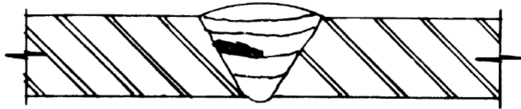
Example of Lack of Fusion Between Weld Passes (B31.3 §341.3.2)
