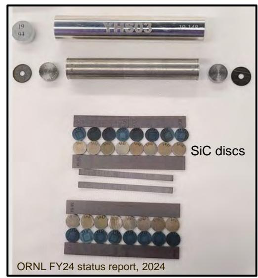
Each capsule holds 16 disc-shaped samples and 8 SiC thermometry (TM)
