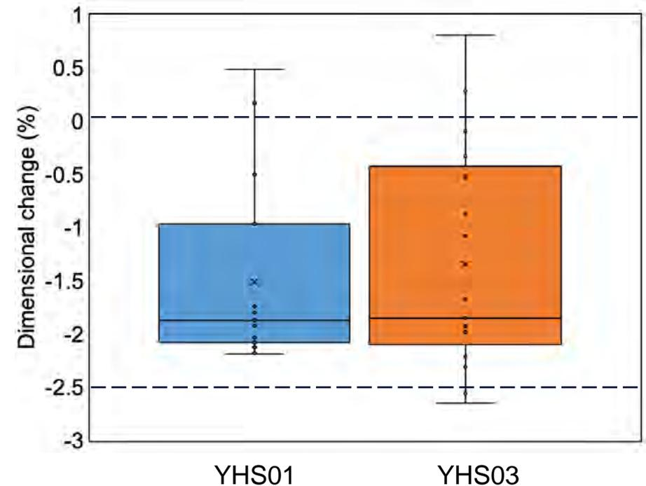
Overall Specimens Tend To Shrink → Density Increase → It Is Not Directly Related To H Retention → MRP PIE Results
