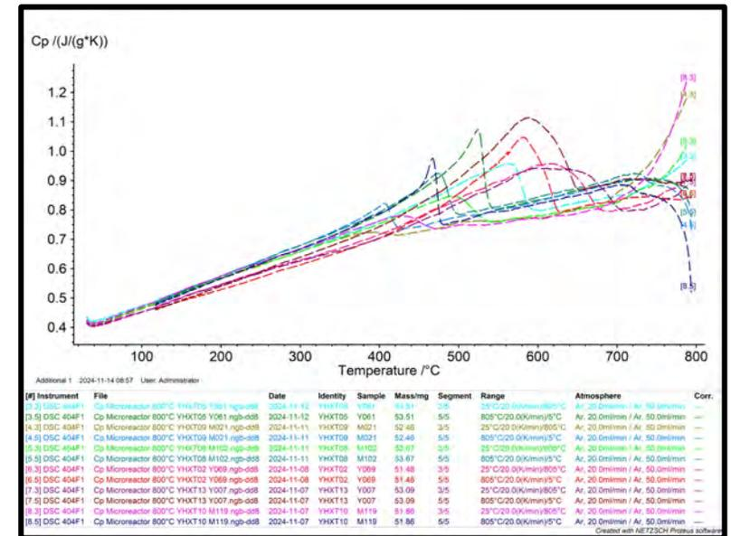
There is  $\Delta T$  between heating and cooling transition temperatures which is directly related to H/Y ratio, thus H retention
