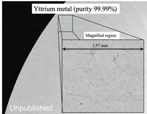
Starting Y (99.99% TREM) metal Main impurities were  $\text{CaF}_2$ ,  $\text{YOF}$ ,  $\text{Y}_2\text{O}_3$
