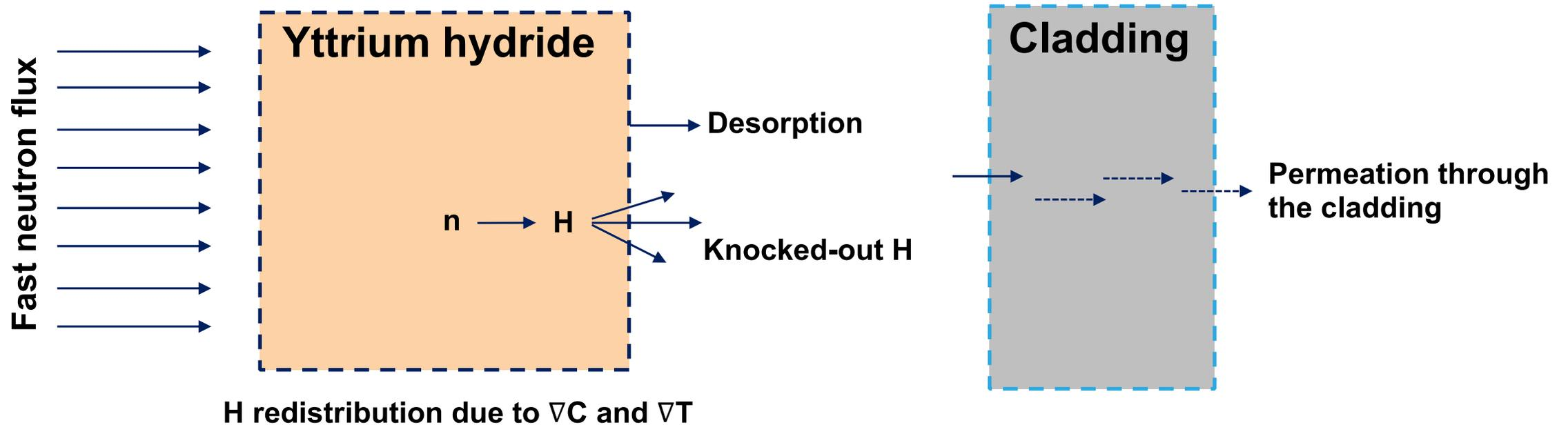
**The Phase Stability Of  $YH_x$  Needs To Be Addressed From The H Retention Aspect Of Hydride-Moderated Microreactors**
