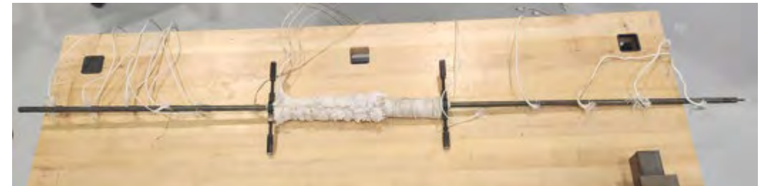
Fig. Instrumentation sodium filled heat pipe
