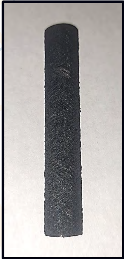
SiC composite shell O.D. : 10.8 mm – 11.2 mm Wall thickness: 0.45 mm Length: 67.0 mm
