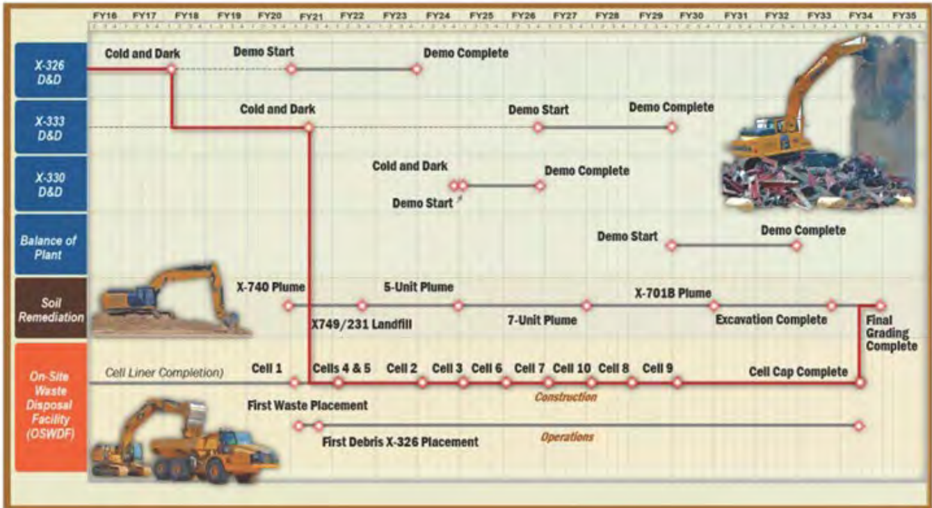
Figure 3-1: Portsmouth D&D Critical Path Summary
