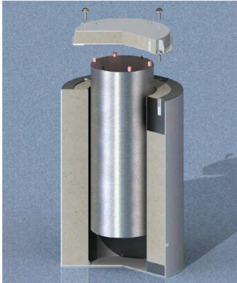
Figure 3-14: Cut-Away View of the HI-SAFE 100 Storage System
