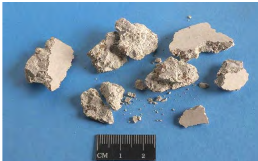
Figure C-4: Typical Debris Resulting from Laser Scabbling of Limestone Aggregate Concrete [1]
