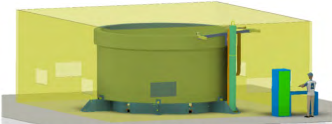
Figure 1 - RAST on Refuel Floor with Modular Containment and RV Ring 1
