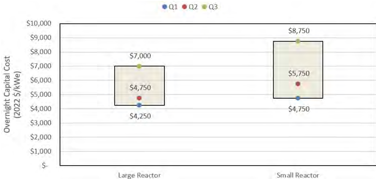
Figure 24. Large reactor and small modular reactor overnight capital costs with contingency removed.
