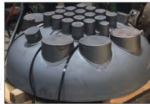
40%-scale, upper head using Powder Metallurgy-Hot Isostatic Pressing (PM-HIP)
