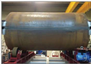
65mm (thick) x 3m length Welding time: < 10 minutes Photograph provided courtesy: TWI (UK)
