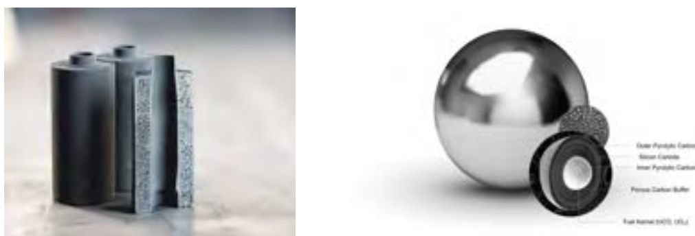
Figure 1: Example of TRISO fuel developed by advanced nuclear reactor companies USNC and X-energy
