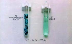
FLUORIDE FUEL FOR A MOLTEN SALT REACTOR
