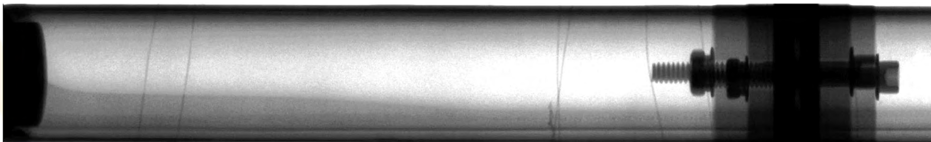
Heat Pipe condenser after heater is shut down: 5x speed, 500 W
