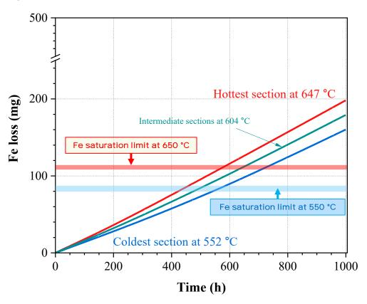
Fe saturation expected in the coldest section after ~600h
