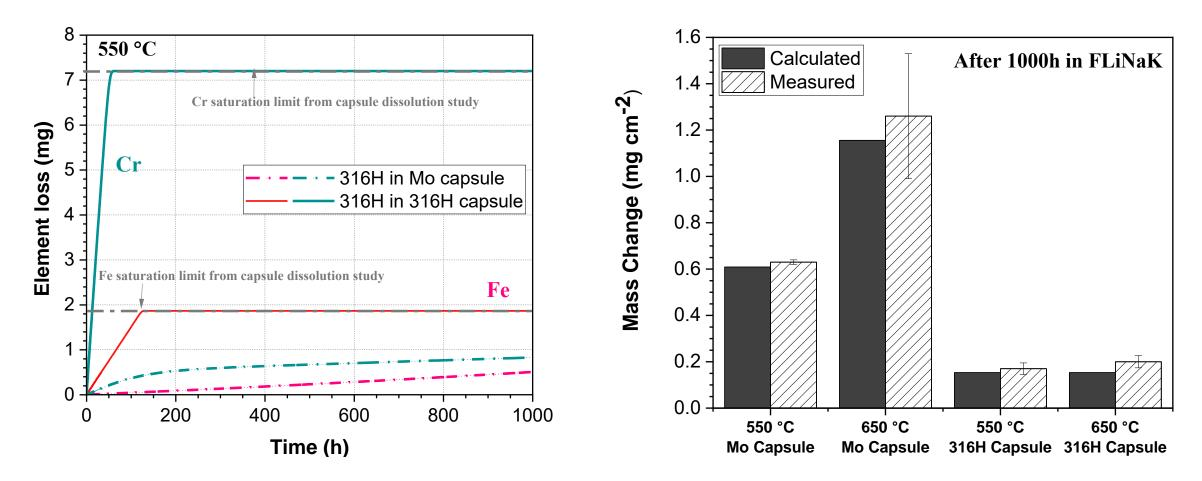
> Saturation limits for Fe and Cr are attained after 48 and 125h respectively for the tests in 316H capsules
