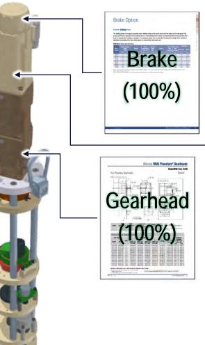
Brake will hold motor torque but may not be needed due to high gear ratio in gearhead series
