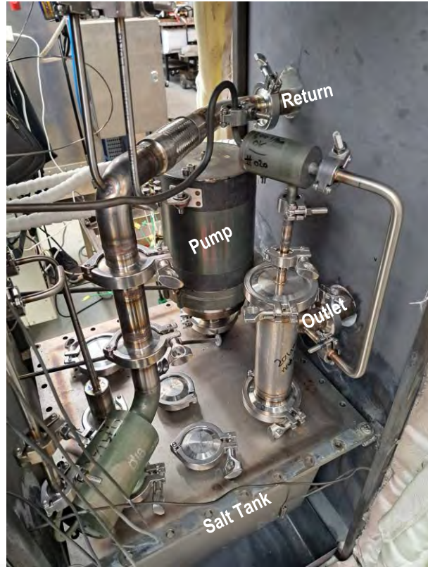
Inside Enclosure Furnace
