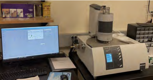
Melting points ( \pm 3 K), enthalpy of fusion ( \pm 3\% for HF DSC, \pm 1\% Calvet), C_p (2% solid and 3% liquid using the Calvet)
