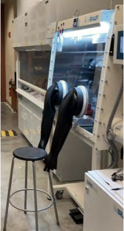
> 40 salts (chlorides, fluorides and iodides) Purification furnace system inside glovebox
