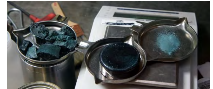
Pu-metal (top), NaCl-36 mol% \text{PuCl}_3 salt (bottom)
