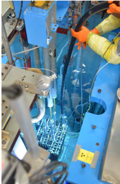
Insertion of experiment in NRAD core on 08/21/2023
