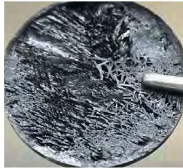
UCl 3 -NaCl salt synthesis performed by Dr. William Phillips (INL)
