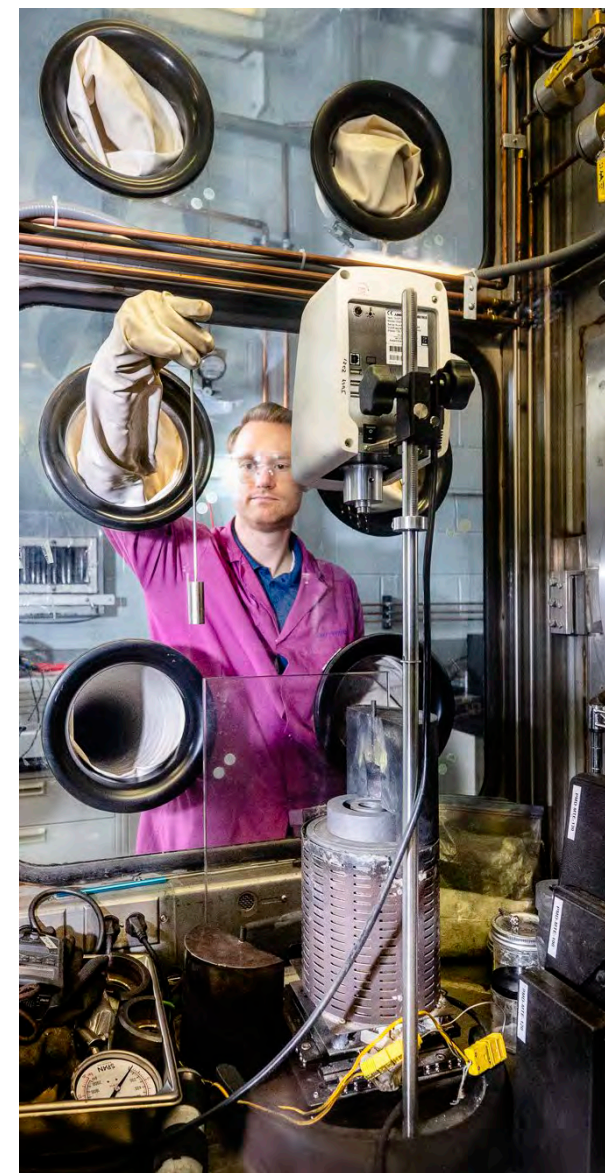
Rotational Viscometer Installed in a Glovebox for Measuring Molten Salt Viscosity
