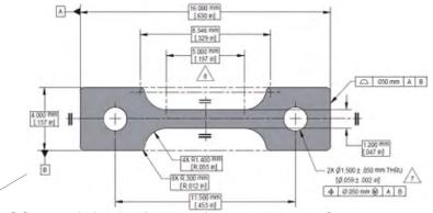
SSJ-3 Mini-Tensile Testing Dog Bone Coupon
