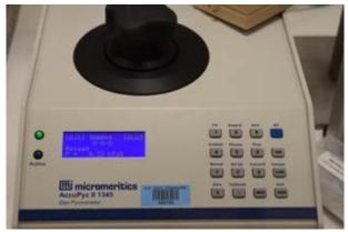
Figure 6. Micrometrics AccuPyc II 1345 gas displacement pycnometer
