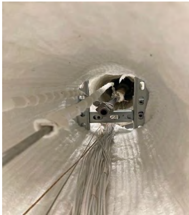
Figure 7. Axial view of the calorimeter coupled to the heat pipe.
