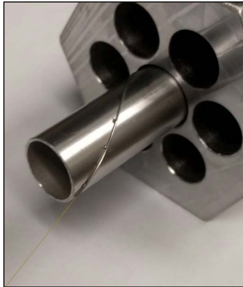
Figure 15. Mockup heat-pipe with fiber-optic wire wrap in test block.
