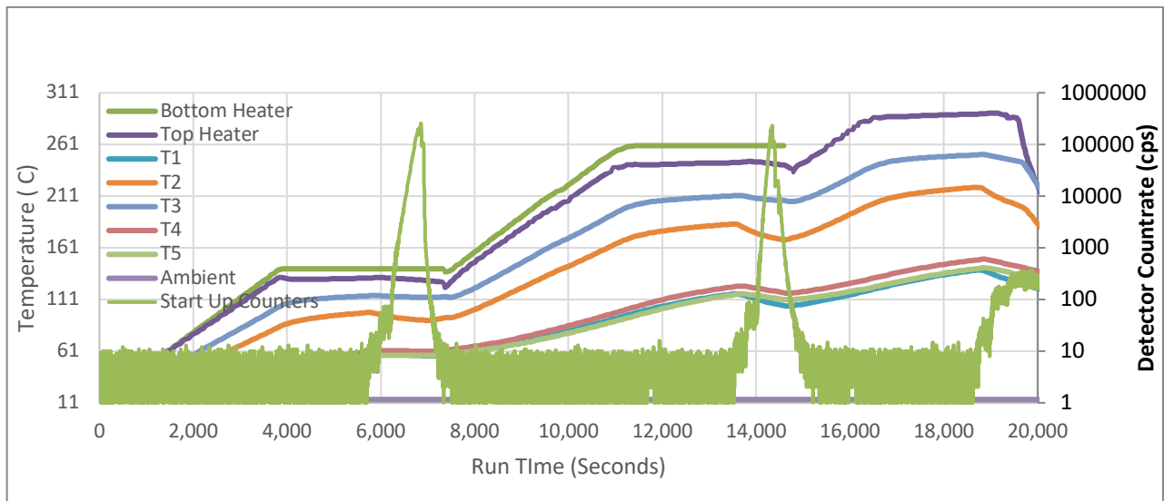
Figure 26. Hypatia Configuration 1 temperature and neutron power profile as a function of run time.
