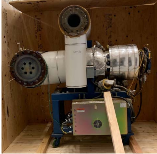
Figure 7. Modified Capstone C30 unit in shipping crate.
