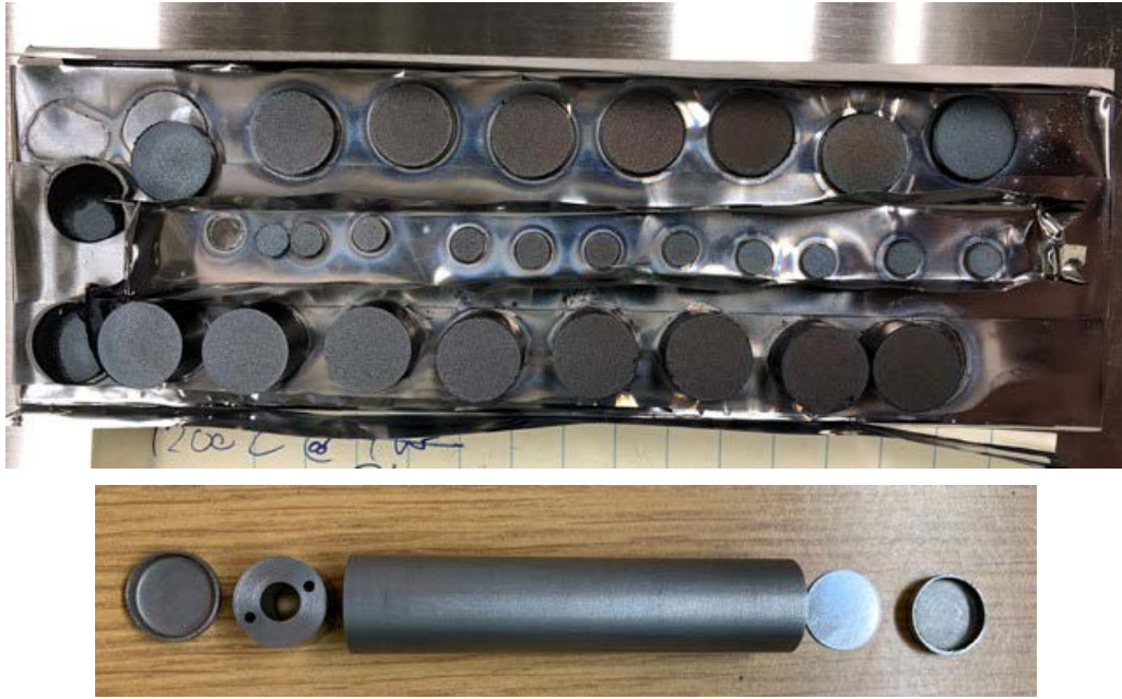
Figure 21. (top) Yttrium hydride samples fabricated for ATR irradiation experiment. (bottom) Tantalum-zirconium-molybdenum alloy (TZM) cans to contain yttrium hydride.
