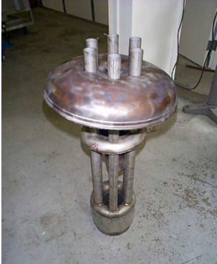
Figure 11. Photograph of Capstone C30 turbine exit dome (top), combustor annulus (middle “dome”), and turbine inlet dome (bottom) with six tubes added by Sandia to transport heater outlet stream to turbine inlet [8].
